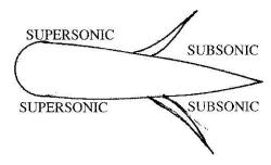
On increasing the speed of the aircraft further the two waves become developed and moves backwards and makes the end of the transonic range. (2 marks)
