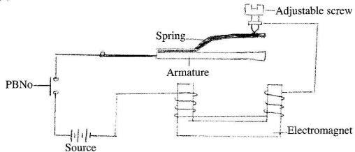
When push button is closed, the circuit is completed.
