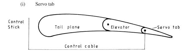
This is the type of tab that is connected to the main control stick to raise or lower the aircraft nose.
