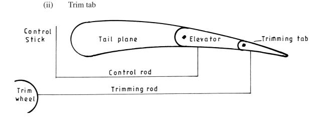
When required say to raise the nose of the aircraft the control stick is pulled backwards. Pulling the control stick lowers the trim tab.
