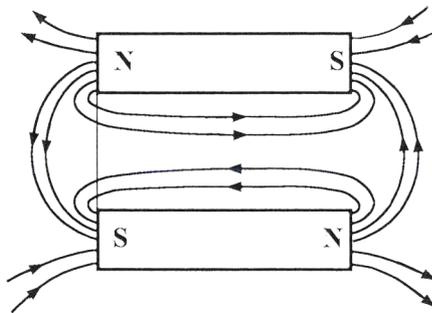
Correct polarity on each magnet
