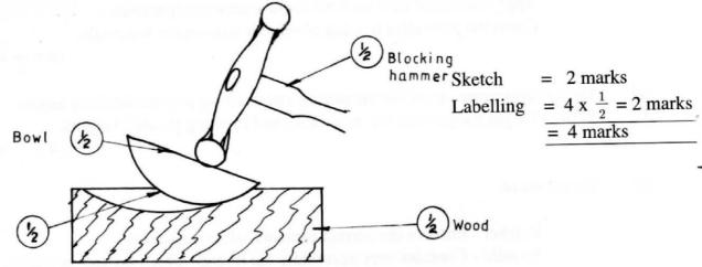
Hollowing on a round block using a blocking hammer.
