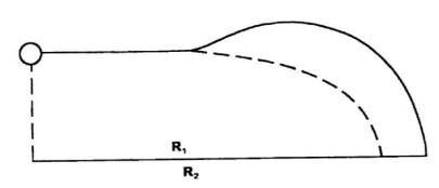
(ii) Spinning causes high velocity of air above  $\sqrt{}$  the ball hence reduced pressure  $\sqrt{}$  which causes the ball to rise higher.
