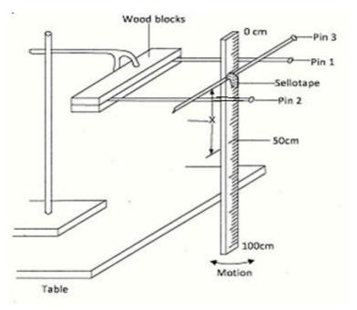
c) Displace the lower end of the metre rule slightly and let it oscillate as shown in the figure above. Measure and record in table below the time t(s) for 10 oscillation (d) Repeat procedure in (b) and (c) above for the values of X shown in the table and fill and complete the table.
