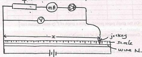
Close the switch and adjust the length x by moving the jockey along the length of the wire mounted on the metre scale till the value of x is 0cm. record the values on the Milliammeter and the voltmeter;
