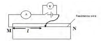
ii. Remove the crocodile clip from the resistance wire MN and close the switch. Record the voltmeter reading V<sub>0</sub>.
