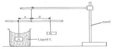
Suspend the mass A at a distance x = 30cm and completely immerse it in liquid L without touching the sides of the beaker.
