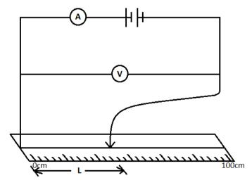
(d) Vary the length by using the crocodile clip along the wire from (when L =0). Record the voltmeter and ammeter readings in the table below. (5 marks)
