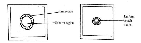
9. The diagram below shows the appearance of two pieces of paper placed in different parts of a non-luminous flame of a Bunsen burner and removed quickly before they caught fire.
