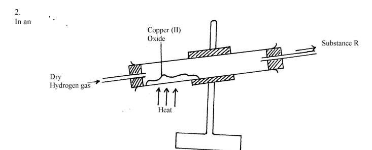
experiment, dry hydrogen gas was passed over hot copper (II) oxide in a combustion tube as shown in the diagram below:-
