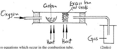
Write two equations which occur in the combustion tube.
