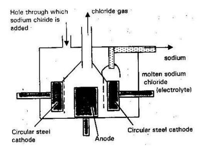
i. What material is the anode made of? Give a reason (2mks) ii.What precaution is taken to prevent chlorine and sodium from re-
