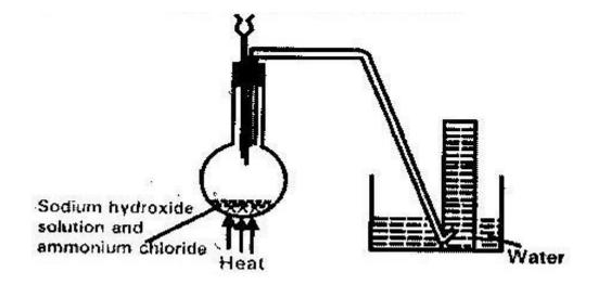
Identify the two mistakes in the set- up represented by the diagram (2 mks)
