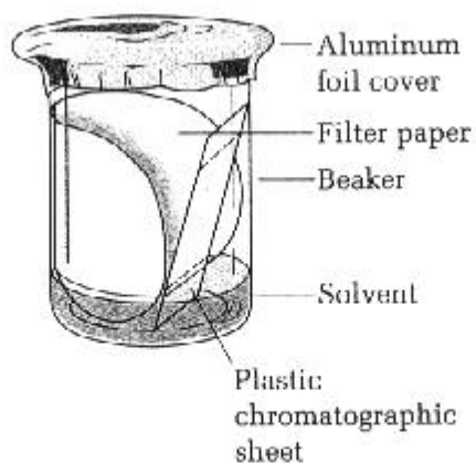
Method used for developing TLC plates
