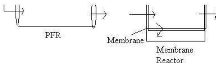
**Fig.4: Schematic Diagram of Plug Flow and Membrane Reactors**
