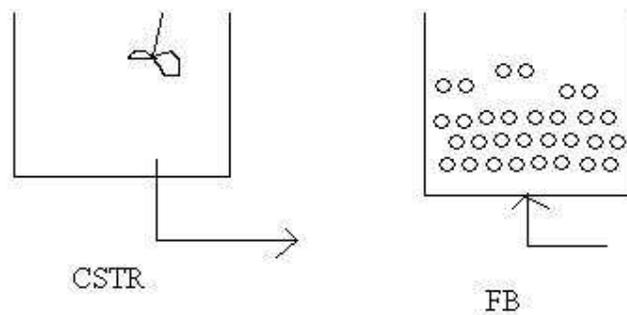
**Fig.3: Schematic descriptions of Continuous Stirred-Tank Reactors (CSTRs) and Fluidised Bed Reactors (FBs)**
