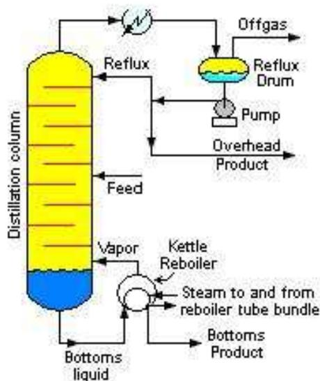
**Fig.2: Diagram of a Typical Industrial Distillation Tower**
