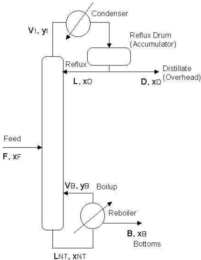
**Fig.1: Schematic Representation of the Operating Principles of Distillation**
