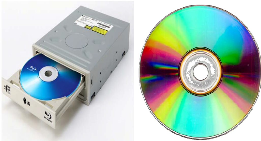
Figure 6.1 A WORM Optical disc. Source: (Google Images, 2009).
