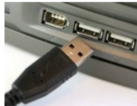
Firewire port (left)
