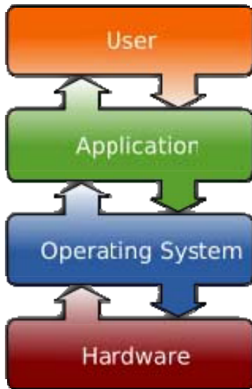
Figure 1.1: A layered structure showing where operating system is located
