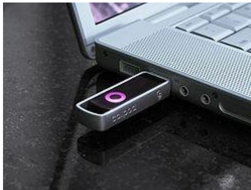
Figure 1.3: A Bluetooth USB dongle with a 100 m range. The MacBook Pro shown also has a built in Bluetooth adaptor.
