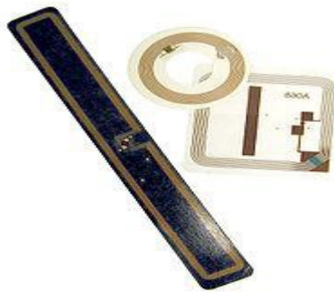
Figure 2.3: RFID tags used in libraries: square book tag, round CD/DVD tag and rectangular VHS tag.
