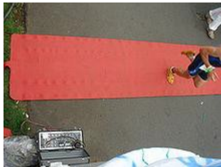
Figure 2.5: J-Chip 8-channel receiver next to timing mat. The athlete wears a chip on a strap around his ankle.
