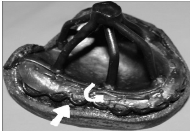
Fig. 4.2: Wax Pattern with Sprues In Situ
