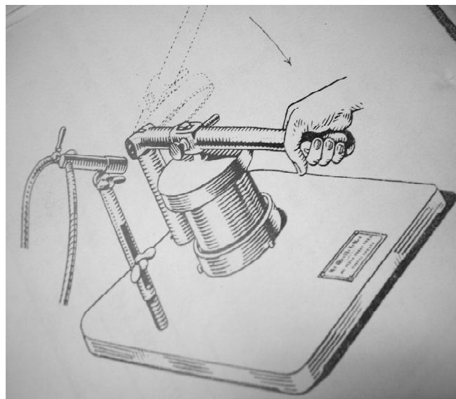
Fig. 2.2: A Solbring Casting Machine
