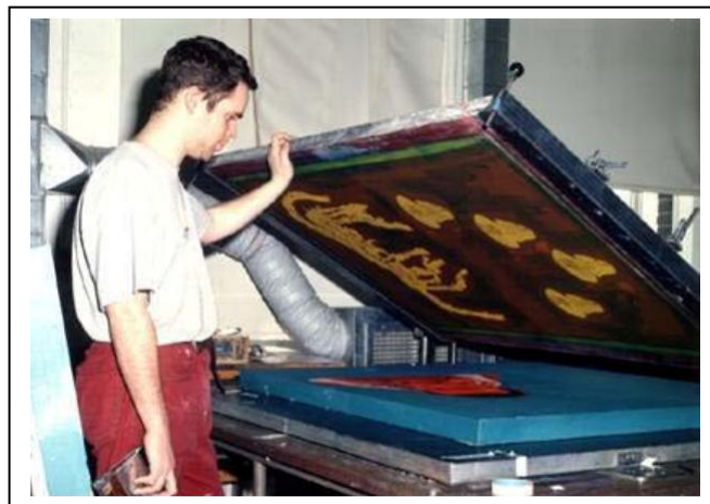
Fig. 38: Silkscreen Printing Source: Microsoft Encarta 2009 .
