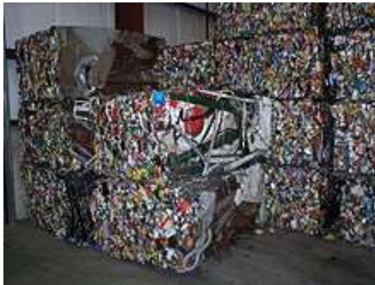
Fig. 5.7: Steel Crushed and Baled for Recycling
