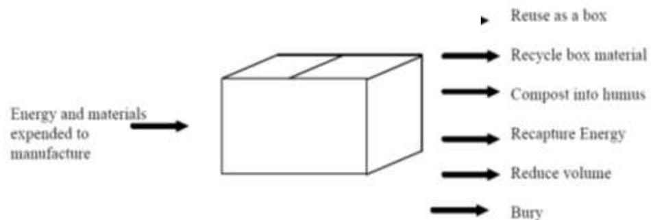
**Fig. 3.1©: Box Potential According to the IWM Hierarchy**
