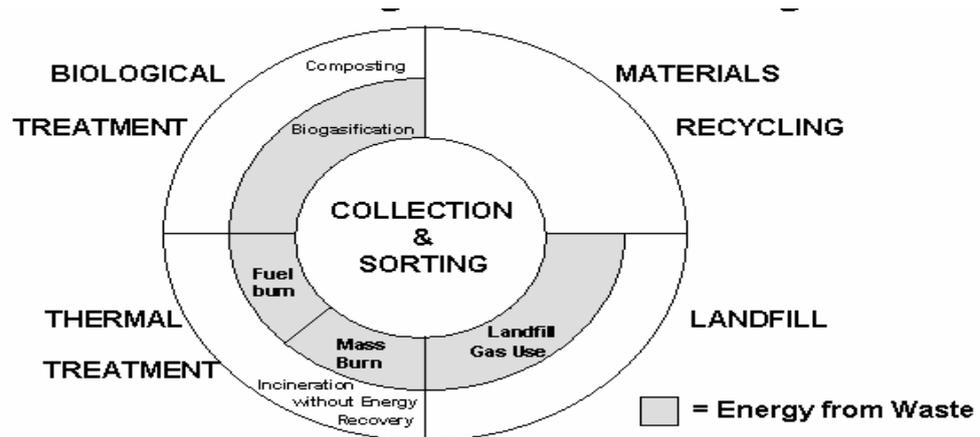
**Fig.3.1 (b): Elements of Integrated Solid Waste Management**
