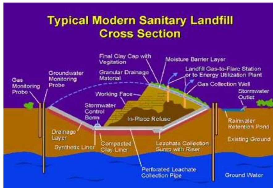
**Fig. 1.2a: Cross Section of a Typical Landfill Operation**
