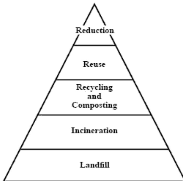
**Fig: 3.1(a): Hierarchy of Integrated Solid Waste Management**
