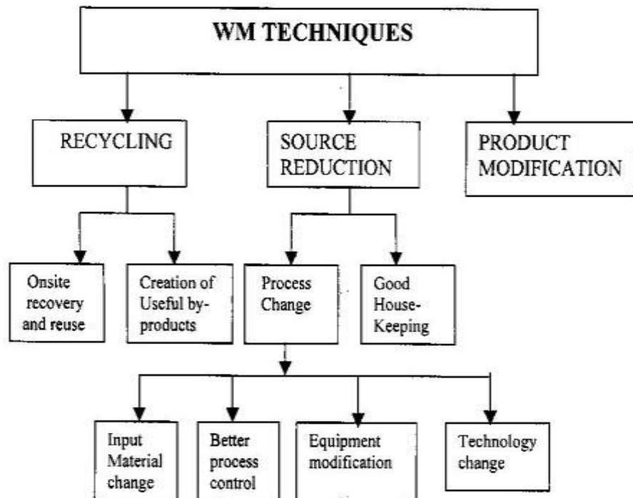
**Fig. 1.1: Schematic Diagram of Waste Minimisation Techniques**
