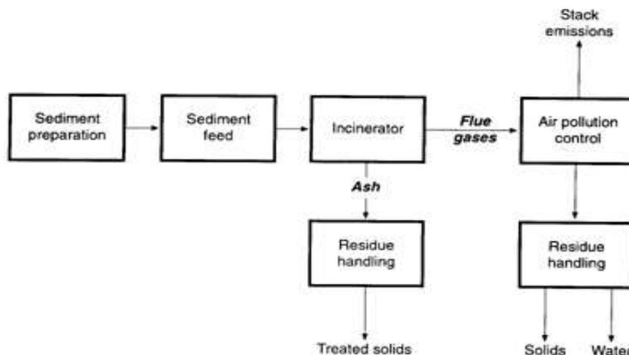
**Fig. 2.1: Diagram of an Incineration Process.**
