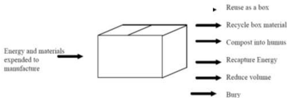
**Fig. 3.1©: Box Potential According to the IWM Hierarchy**
