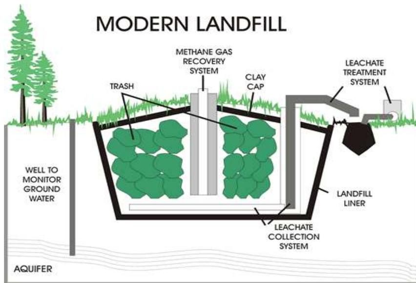
**Fig. 1.2b: Main Features of a Modern Landfill**
