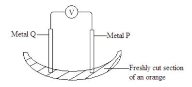
(a) **Show** the direction of flow of electrons on the diagram using an arrow. (1mark)
