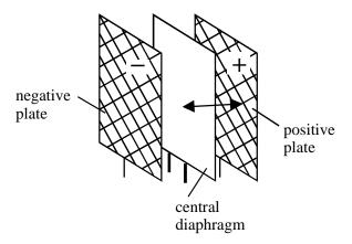
The output from an amplifier is connected to the central diaphragm. This causes the charge on the diaphragm to alternate between positive and negative.
