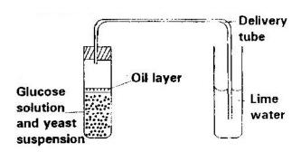
Glucose solution was boiled and oil added on top of it. The glucose solution was then allowed to cool before adding the yeast suspension.
