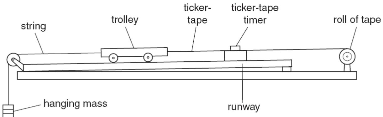
For each mass, hung as shown, the acceleration of the trolley is determined from the tape.
