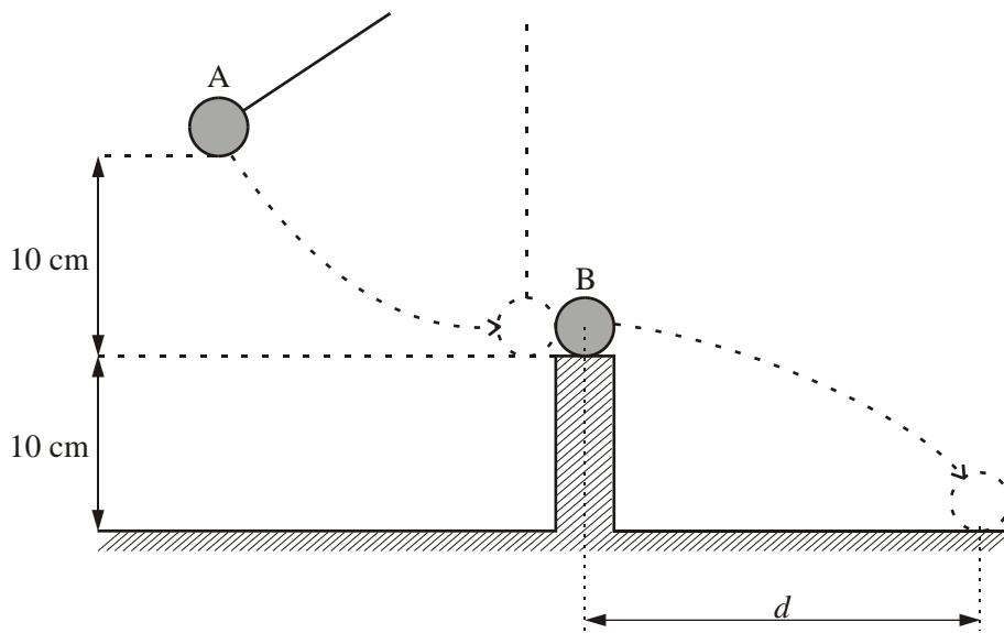
Sphere A is tied to the end of a long vertical thread and pulled to one side until it has risen a distance of 10 cm. It is then released and comes to rest when it strikes the sphere B which is resting on a smooth flat support.
