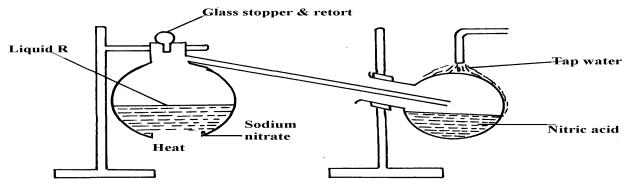
(b) The set-up below was used to prepare nitric acid.
