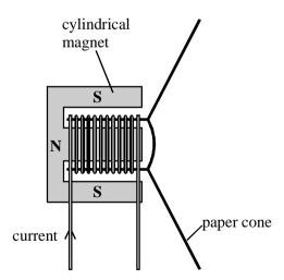
(a) (i) When the current is in the direction shown in the diagram, the paper cone moves to the right.
