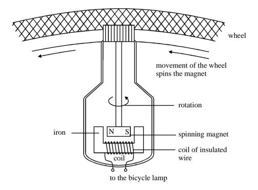
An alternating voltage is induced in the coil when the magnet rotates. The graph shows how the induced voltage changes with time for half a revolution of the magnet.
