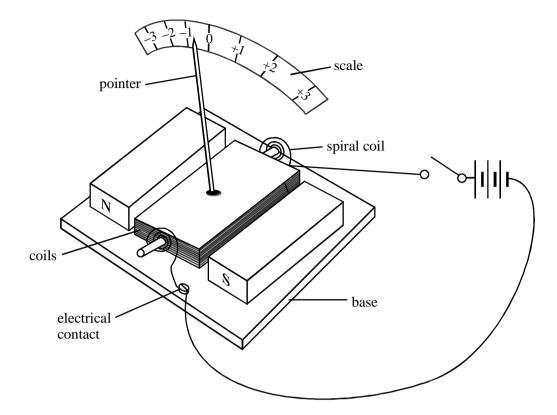
When the switch is closed, the needle moves to the point +3 on the scale.
