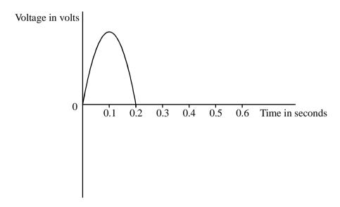
(i) Continue the graph to show the voltage as the magnet turns through a further half revolution.
