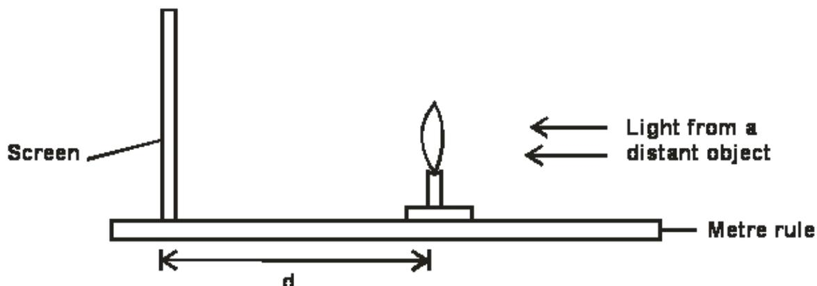
b) Adjust the distance of the lens from the screen until a well-focused image of a very distant object like a tree, is seen on the screen. Record the distance between the screen and the lens as  $d$ .
