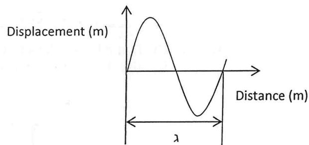
From the information above show that the speed of the wave = frequency  $\times$  wavelength
