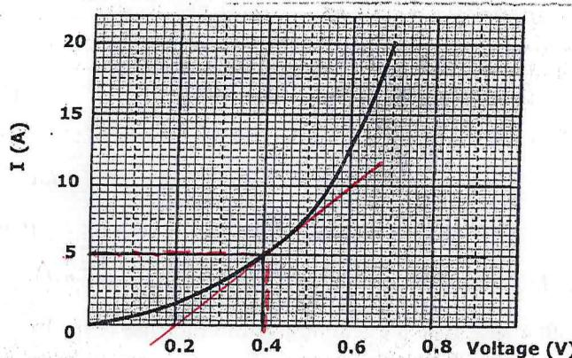
(i) From the graph, determine the resistance of the lamp when a current of 5A flows. (3 marks)
