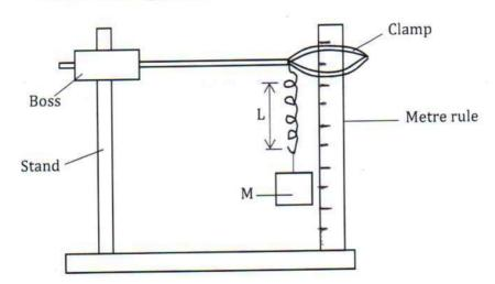
(ii) Measure the length  $L_0$  of the unloaded spring.
