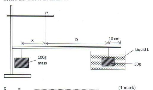
Apply the principle of moments to determine  $W_2$  of the 50g mass in the liquid L and hence determine the upthrust  $U_L$  in the liquid. (2 marks)
