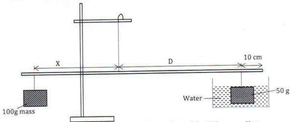
The balance point is attained by adjusting the position of the 100g mass. Note that the distance X and D are measured from the supporting string and the 50g mass is fully submerged in water.
