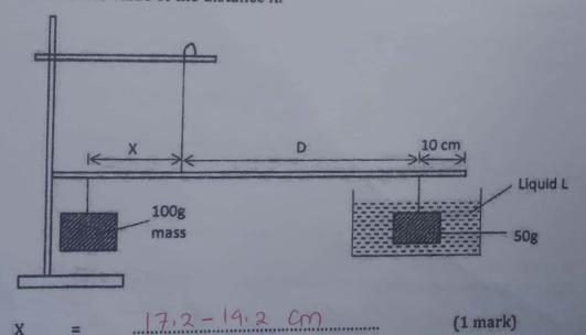
Apply the principle of moments to determine W2 of the 50g mass in the liquid L
