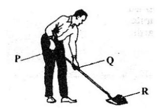
Which one of the following positions labeled **P**, **Q** and **R** represent the load, effort and fulcrum when the machine is in use?
