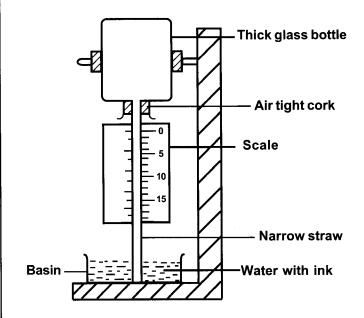
When it is placed in a hot sunny weather, the instrument did not work. What mistake was made?
