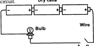
Which of the following materials cannot be placed at the gap marked AB to make the bulb light?
