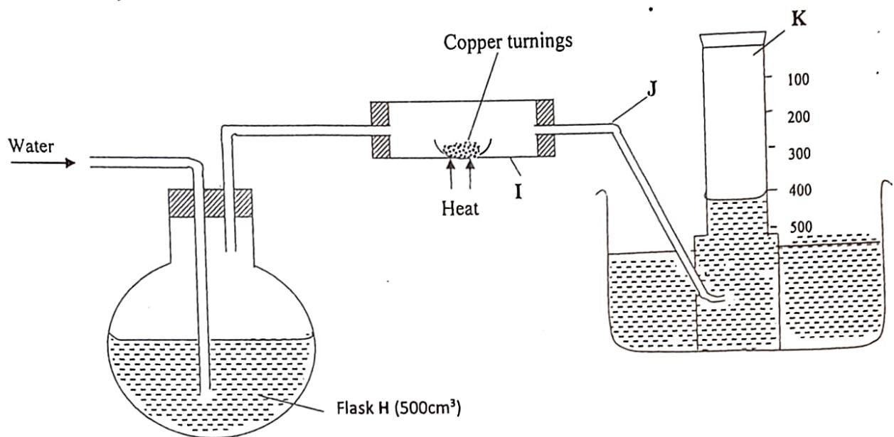
A  $500\text{cm}^3$  measuring cylinder K was filled with water and assembled for gas collection. Copper turnings were heated red hot and water was slowly passed into  $500\text{cm}^3$  flask H until it reached the  $500\text{cm}^3$  mark. A colourless gas was collected in K.
