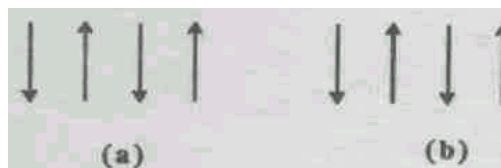
Fig. 5.4 Relative orientation of electron spins in (a) antiferromagnetic material and (b) ferrite.
