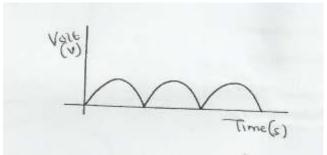
(ii) During the first half-cycle D<sub>1</sub> is forward biased while D<sub>2</sub> is reverse biased. Hence, current takes the path A, D<sub>1</sub> RT. During the next half-cycle, D<sub>2</sub> forwarded biased while D<sub>1</sub> is reverse biased and the path of the current is BD<sub>2</sub>RT.
