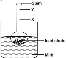
i) The upper stem of a hydrometer is made thin. Give a reason for this.
