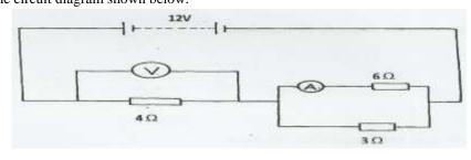
(ii) Determine the reading of the voltmeter V.
