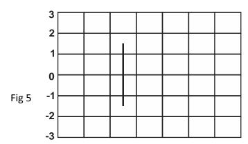
If sensitivity of the Y-gain is 30V/division, find the voltage of the signal.
