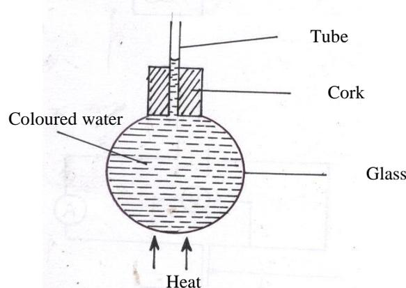
*Glass flask expands first, creating more volume for water ✓. Water then expands increasing its level in the tube ✓*
