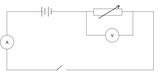
b) Adjust the potentiometer until you are able to obtain minimum reading on the voltmeter and maximum on the ammeter. Record these readings in the table below.
