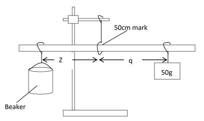
Use the cello tape provided to fix the position of the 50g mass. Note the point of suspension must remain the same throughout the experiment.
