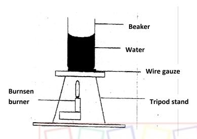
Measure 100cm<sup>3</sup> of water and pour it into the beaker. Take the initial temperature of the water.
