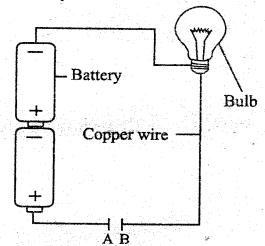
Which of the following materials will not make the bulb light if put between A and B?
