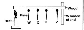
After sometime the pins dropped starting with **W** to the last pin **Z**. This was due to transfer of heat through a process called
