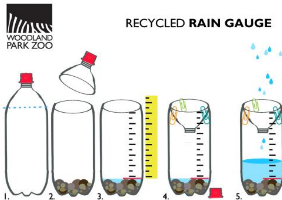
Figure 5.1: Procedure for construction of improvised rain gauge adopted from Indian Weatherman.
